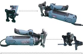
Jigsaw with a bevel function on the sole part allows cutting angles of typically up to  $45^{\circ}$  relative to the normal vertical stroke for cutting mitre joints: Jigsaw also can cut in a rapid up and down motion. The key to excellent result with a Jigsaw is to match a specific blade to the type of material that you'll cut: wood/metal/plastic
